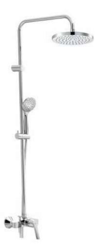
Shower mixer with Dual shower system L-shape L = 1175 mm wall fastening hand and head shower with divertor with 1S hand held shower 1/2 inch ridgeless adjustable shower holder vertically and cylindrically adjustable shower holder shower hose 1/2 x 1/2 inch x 1600mm with fixing kit swivel head shower
