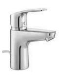
Single lever basin mixer DN 15 ceramic cartridge - K35 aerator M 24 x 1 1/2" high pressure flexible hose with PEX tubes pop up waste 1 1/4 inch European Standard- EN 817
